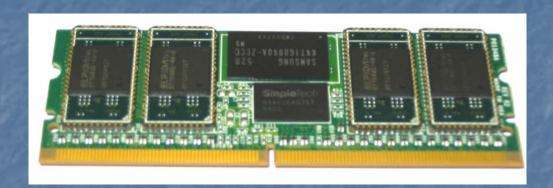
82mm versus 133mm = 40% reduction in size versus full size RDIMM
